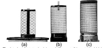
Figure 1. The interior of a tetrode: (a) mesh filament, (b) control grid (c) screen grid
