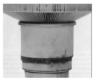
Figure 6. An industrial triode that failed because of socketing problems.
