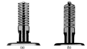
Figure 3. 5762/7C24 spiral filaments: (a) normal filament, (b) abnormal filament
